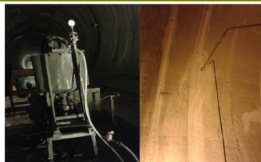
Photo: Arrangement for water percolation test- Grout pump, Pressure gauge, Water meter, Packer and pipes.
